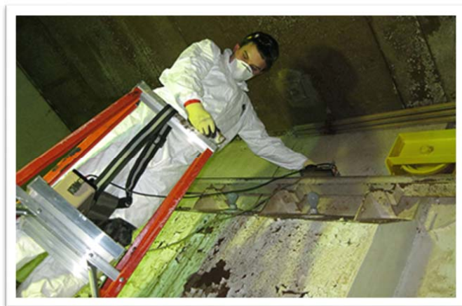
Slika 4.3 Radiološka prospekcija zidova u nuklearnom objektu, https://www.orau.org/environmental-assessments-health-physics/success-stories/georgia-tech-neely-research-center.aspx
